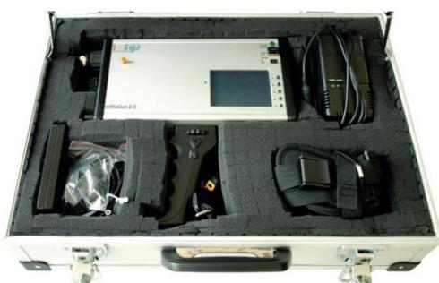
For plastic identification the unit is just held on the surface of the sample and measuring starts by pressing the trigger button. Single measurements can be made as well as online measurements with a fixed trigger key – like for the quality control of mixed granulates etc.
