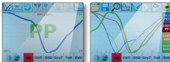
The new **mIRoGun 2.0** measures plastic and textile parts of all kinds and types as diffuse Near Infrared Reflection Spectrometer with completely new hard- and software at a very high speed. The samples can be solid parts, films and foils, granules, fibers or foams.
