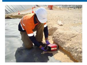
RemScan is used to monitor the soil after remediation to ensure that it complies with site requirements. For bioremediation processes, RemScan can monitor the decrease in the concentration of the contamination over time to determine the end point. Once the soil is "clean", it can be removed from the bioremediation pad, thereby increasing the utilisation and throughput of the bioremediation facility.
