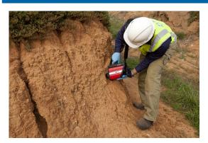
While excavation work is being performed, RemScan can measure the remaining soil to check whether all of the contaminated soil has been removed and whether the remaining soil is clean. Once all contaminated soil has been removed, samples can be sent to the laboratory for final auditing and statutory signoff.
